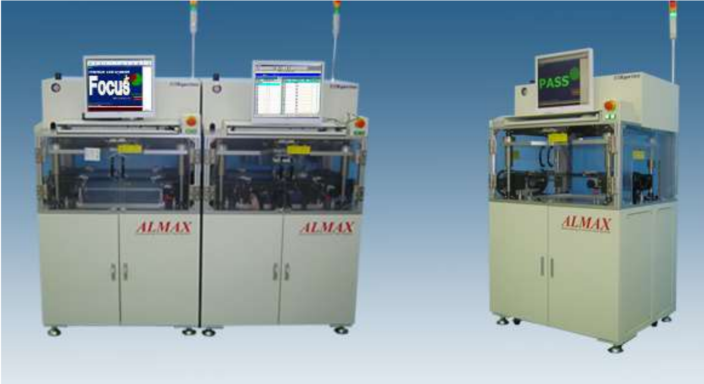
(Left)In-Line Full Automatic ICT&FCT integration / (Right) In-Line Full Automatic ICT
