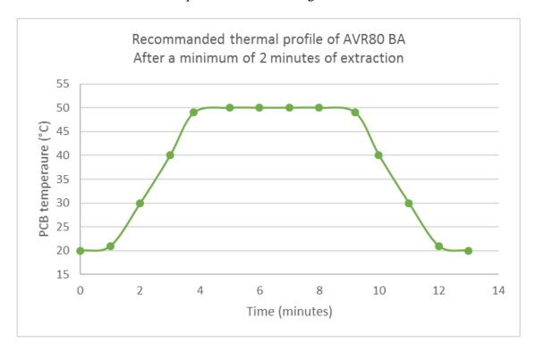
This thermal profile can be adapted:  $\pm 10^{\circ}$ C, depending some more parameters, such as: thickness deposit, design of the PCB...
