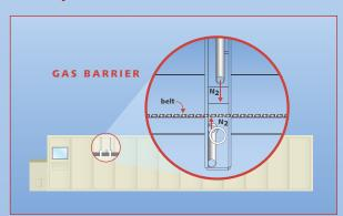
The Controlled Atmosphere Furnace from BTU features precise atmosphere controls to monitor critical parameters within the process chamber. The gas control panel is designed to operate in a safe/ failsafe manner while minimizing operator intervention.
