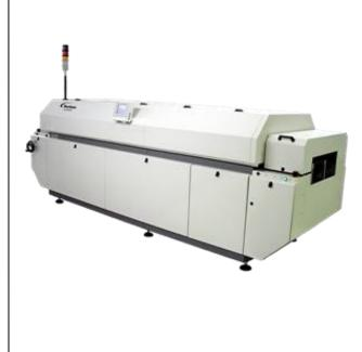
The in-line Thermal Cure oven is ideal for mid-tohigh volume production and is designed for easy integration with all Nordson ASYMTEK conformal coating systems. The CE-compliant oven features precise control of conveyor speed and internal thermal environment. Infrared panels and exclusive heat dispersion plates transfer heat by convection.
