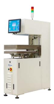
The FlexTRAK-S platform handles a wide variety of product form factors, including boats, carriers, Jedec/Auer® boats, strips, and laminates. Depending on throughput and product form requirements, the system can be configured for magazine-to-magazine processing of single and multiple strips or lead frames and standalone for island-based production environments.
