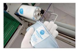
World leading Teknek Nanocleen  $^{\text{TM}}$  cleaning core. Nanocleen  $^{\text{TM}}$  is a silicone and static free system that is capable of cleaning particles smaller than 1 micron. Ideal for thin, sensitive materials such as polyimide, polyester, copper etc.
