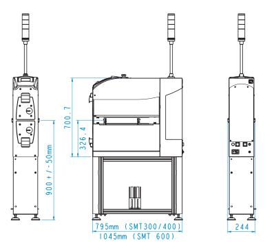
*Note:* The standard SMT clean machine has a cleaning width of 400mm. It is also available with a cleaning width of 300mm and 600mm.
