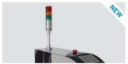
The staged Alarm Beacon ensures at all times that the operator is aware of the running condition of the machine. The ability for the customer to adjust the height of the beacon is possible, ensuring consistency along the line. Volume control is also a standard feature on the beacon.
